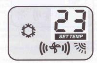
If the air sensor built in the Room Control is enabled, the display after few seconds will indicate the room temperature.
