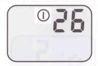
(): OFF The unit will not control the room temperature at all if the Room Controller is operating in an "() off" period.
