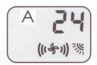
A: AUTO "auto" Heat / Cool is used to control a room temperature set point automatically.
